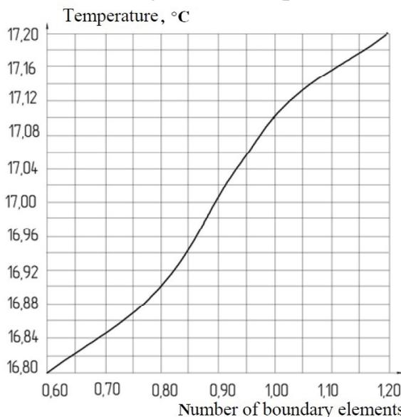
Fig. 3. Temperature distribution, depending on the number of boundary elements
