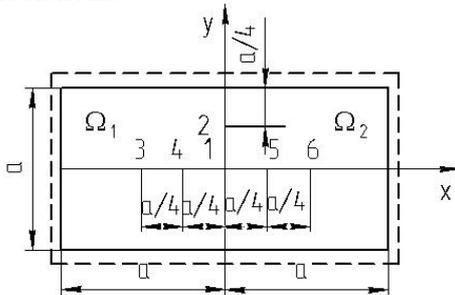
Fig. 6. Rectangular plate consisting of two areas
