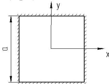
Fig. 2. Square plate that is pinched in the contour under the action of a uniform load
